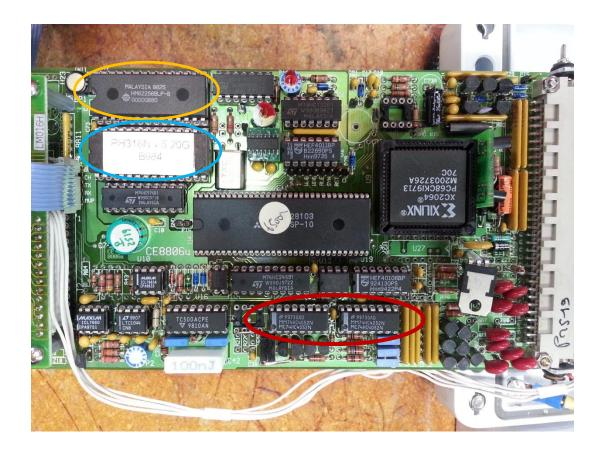
If the instrument is showing strange internal voltage, *example* !!!! or higher than normal readings check these IC multiplexers by switching them. If internal voltage show normal after switching, replace both.
